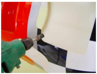
3. Use templates to cut out other openings in the cowl for manifolds if fitted.
