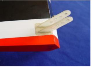
6. Make sure the horns are correctly aligned (by installing the linkage bolt) before the epoxy has cured.
