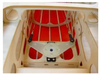
NOTE: The pull-pull connector is only threaded half way into the ball link to allow for final adjustment.
