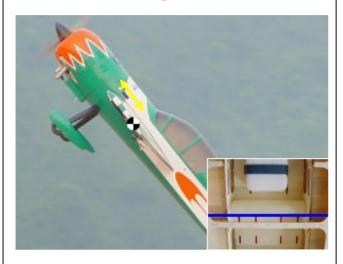
Your balance at the CG will determine the fin al mounting location for batteries. Mount batteries and secure with Nylon zip ties
