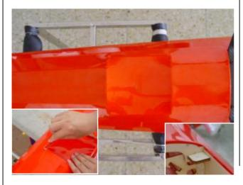
2. Epoxy the bracket in place supported by triangular hardwood supports.
