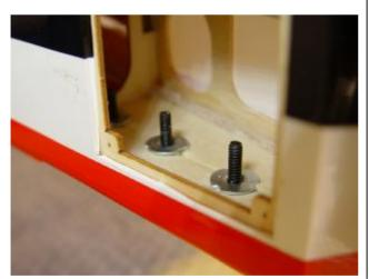
4. Install the hatch with 4 screws using the pre marked screw holes.
