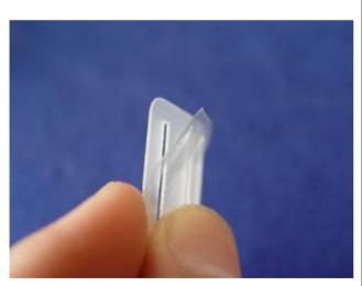
2. Trace around the locking plate with a knife and remove the covering below to expose the pre-cut slots.
