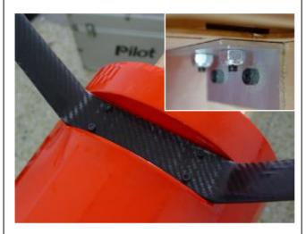
2. Install the landing gear axles with lock nuts but do not tighten yet.
