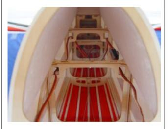
3. Install servos as shown with the servo label facing the rear of the fuselage.
