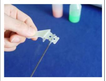
5. Fit the horns into the locking plate and then insert them into the pre-cut slots. Align the right and left sides before the epoxy cures. Wipe away excess epoxy with rubbing alcohol
