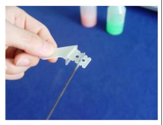
5. Fit the horns into the locking plate and then insert them into the pre cut slots. Align the right and left sides before the epoxy has cured. Wipe away excess epoxy with
