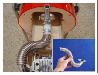
2. Tighten the manifold bolts and secure with Blue Loctite.
