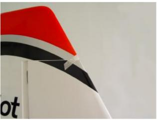
3. Attach the pre-installed bolt link to the rudder horns without locking nut as shown.
